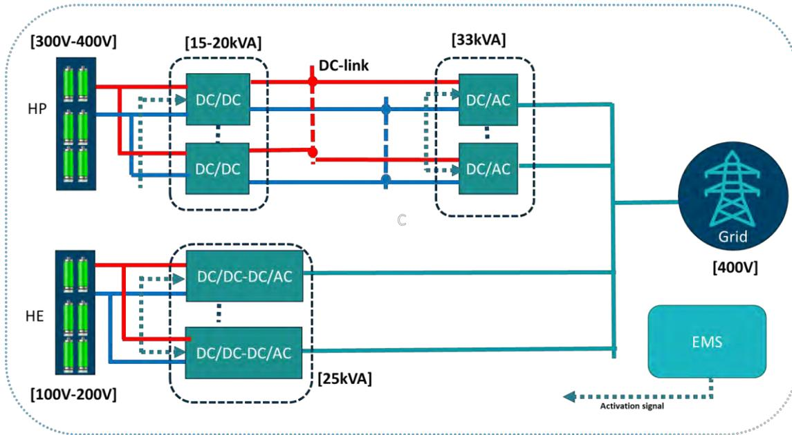
Figure 7. PE configuration 4: interface 1 for HE pack and interface 2 for HP pack
