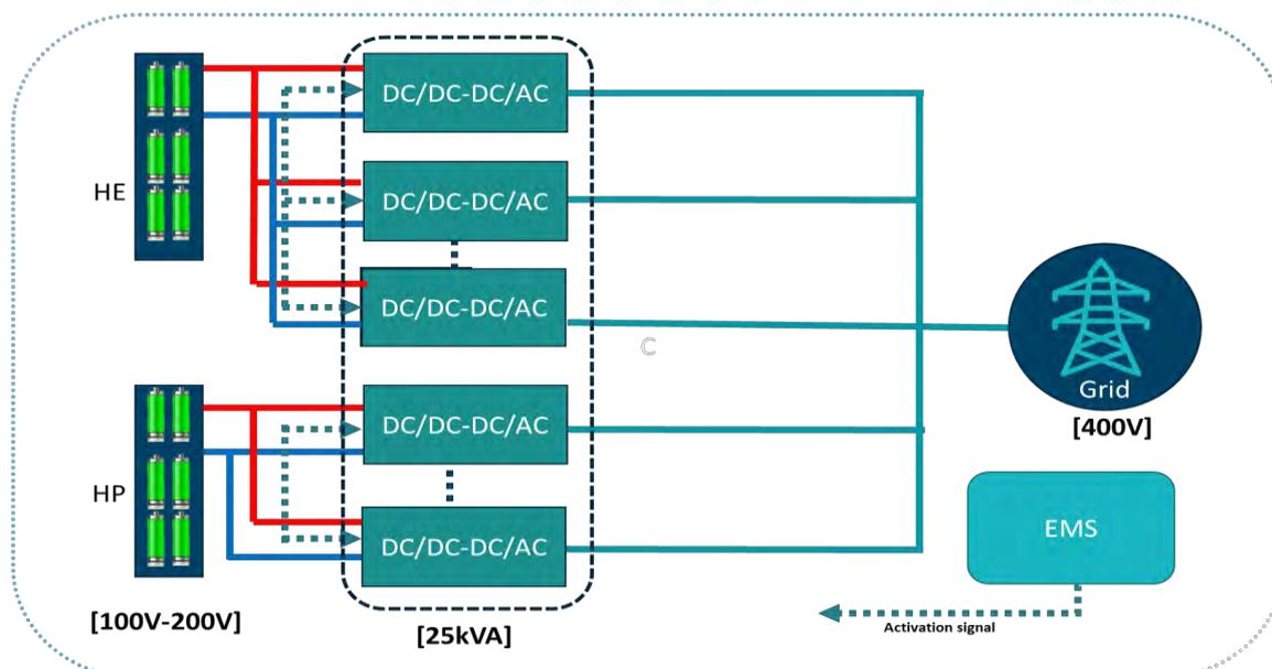
Figure 4. PE configuration 1: interface 1 is used for HE and HP packs
