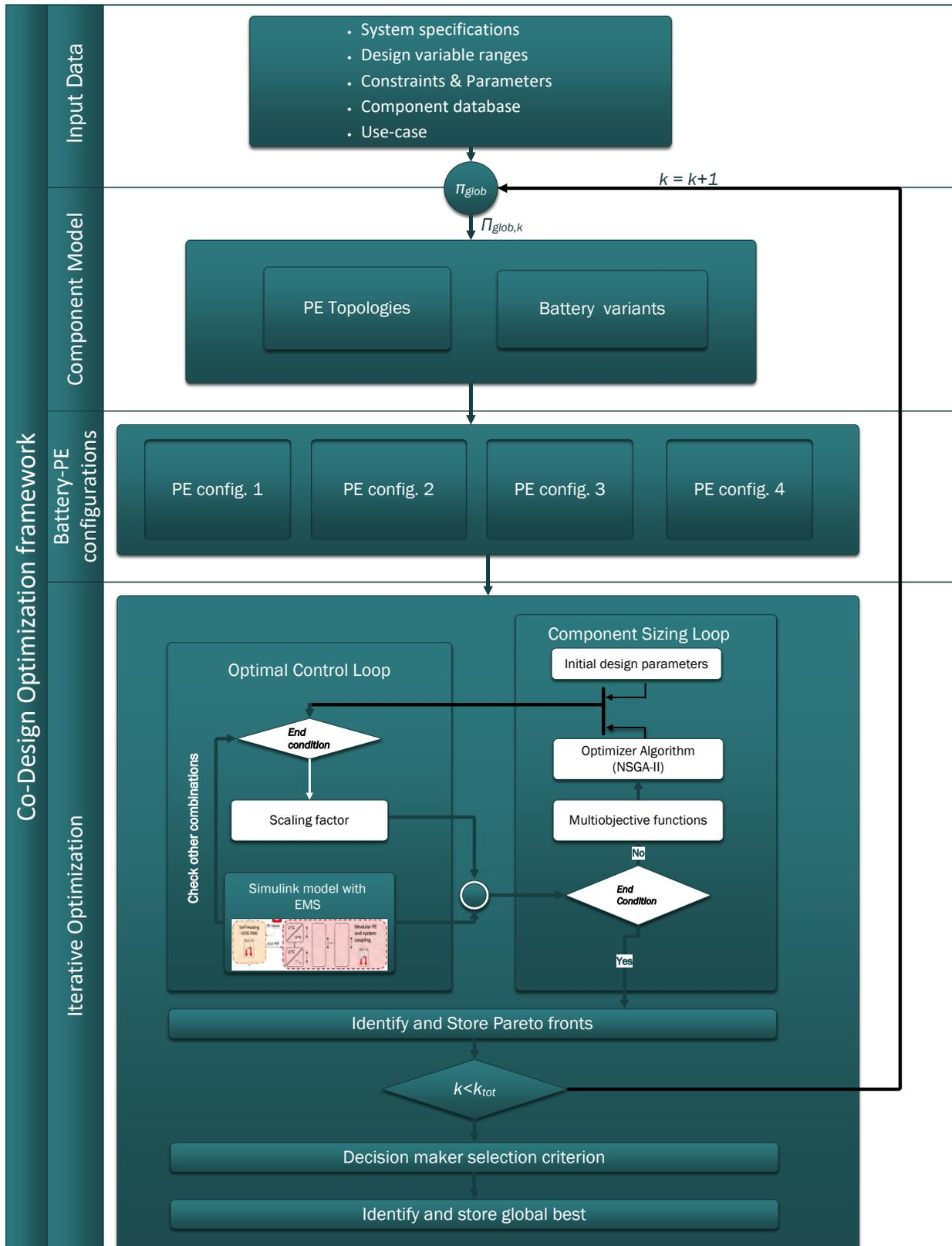
Figure 14. Co-design optimization framework architecture
