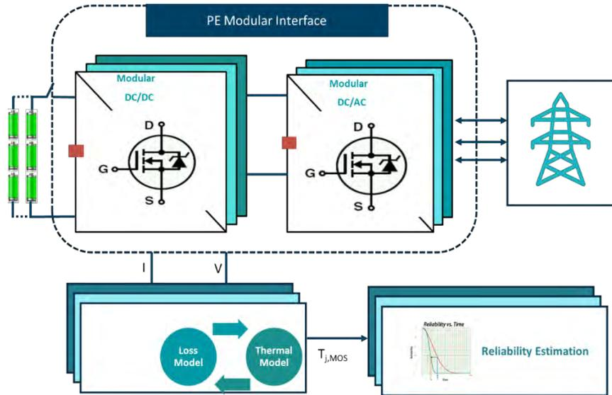
Figure 11. Lifetime estimation process from the LoFi model of the PE interface
