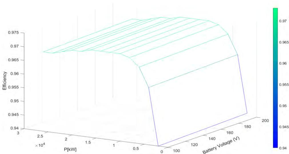
Figure 8. Efficiency map for 1 module from OEM1 comprised of a single stage DC/AC
