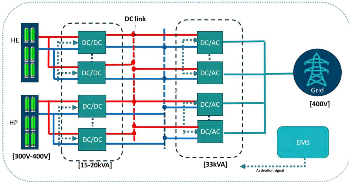
Figure 5. PE configuration 2: interface 2 is used for HE and HP packs
