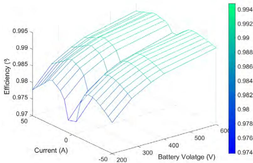
Figure 10. Efficiency map for 1 DC/DC module from OEM2
