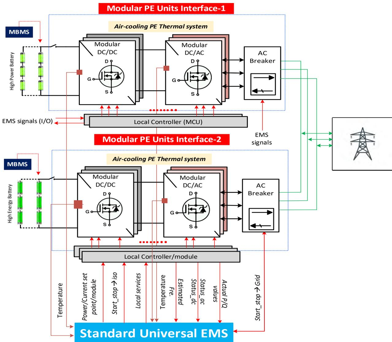
Figure 2. Overall system architecture of the Modular PE interface with both logical (red) and physical (black) interface connectivity (D1.1)
