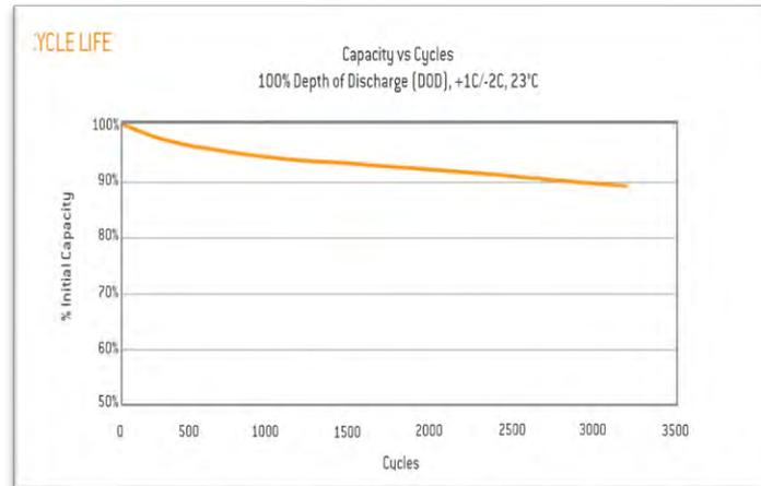
Figure 3. Cycle life characteristics of an A123 cell [3]
