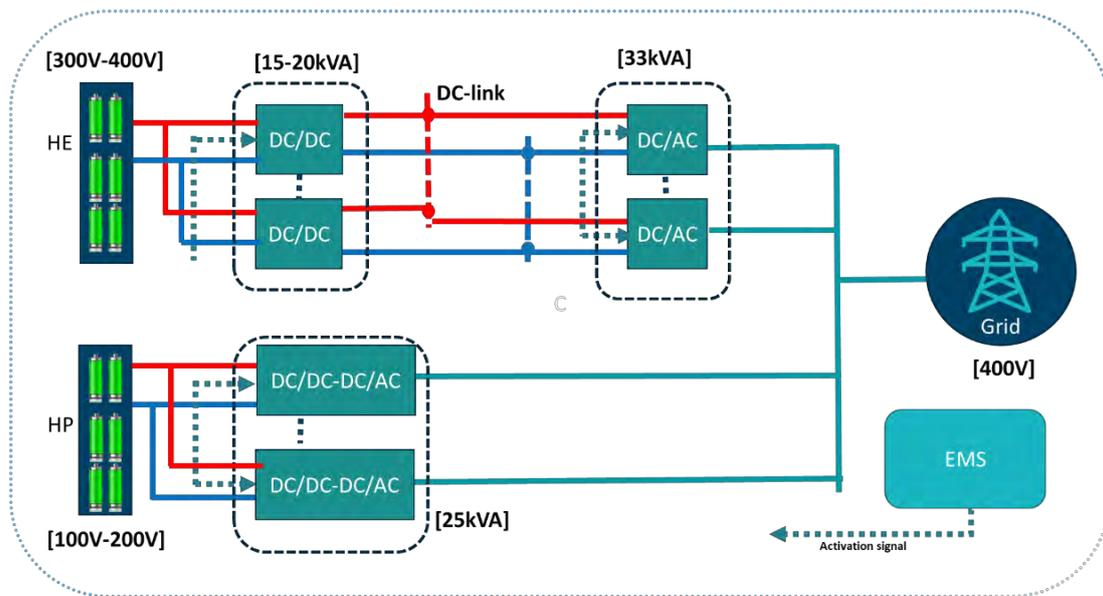
Figure 6. PE configuration 3: interface 2 for HE pack and interface 1 for HP pack
