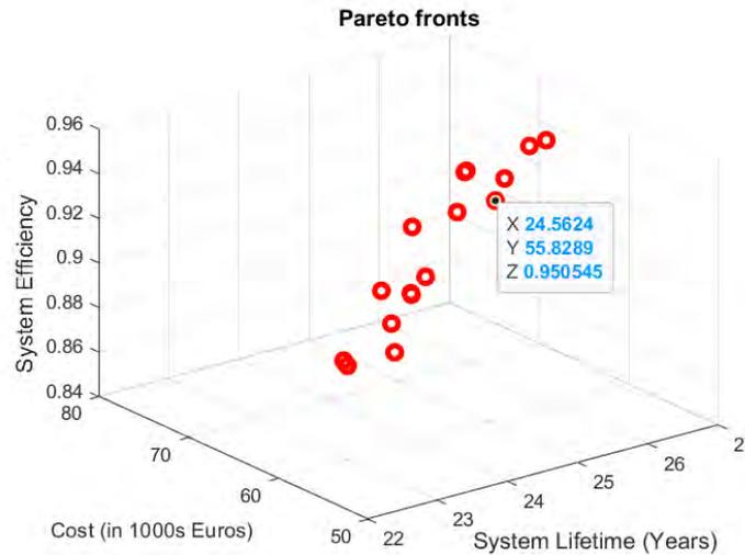
Figure 15. Feasible solutions with LFP and LTO cells connected with PE interface 1
