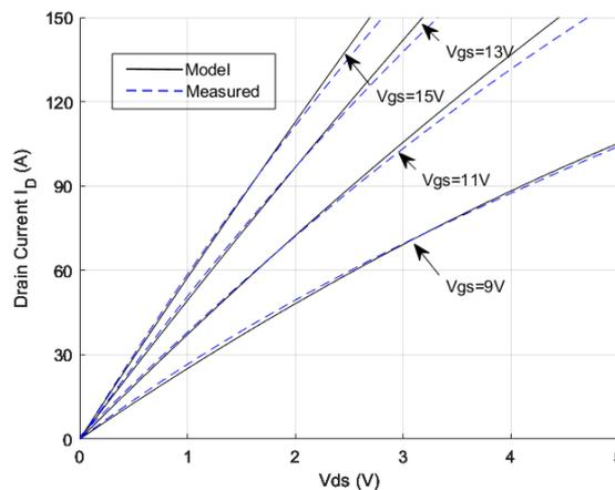
Figure 17. Static performance with relation to drain current, drain voltage and different gate voltages at 25°C
