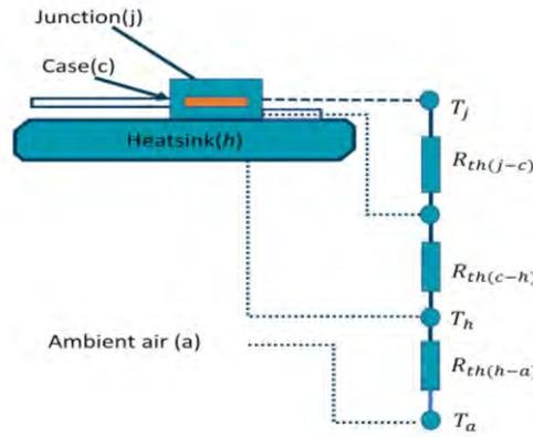
Figure 13. Thermal profiling approach for switch modelling.
