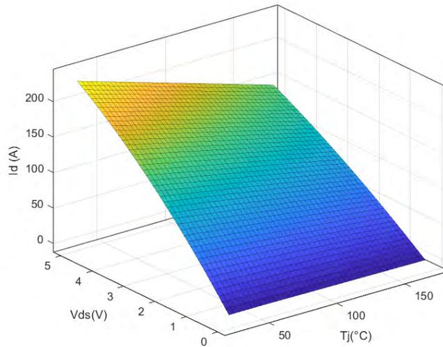
Figure 18. Drain voltage-current behaviour at different junction temperatures.
