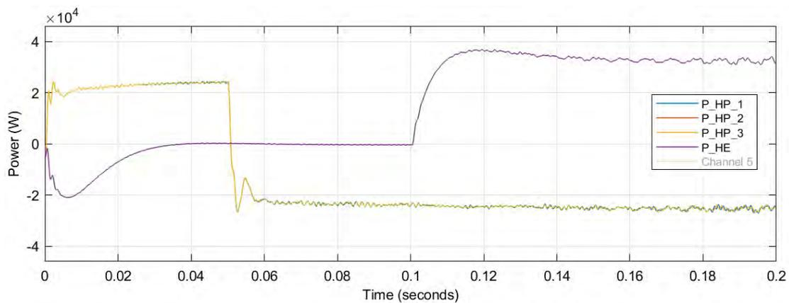
Figure 25. Exchanged active power of the entire converter topology
