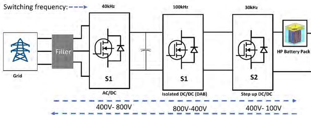
Figure 4. PT PE interface connecting the HP battery pack to the grid.
