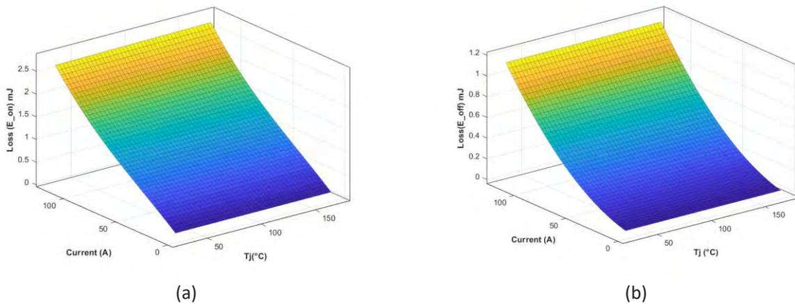
Figure 19. ZIG semiconductors switching losses
