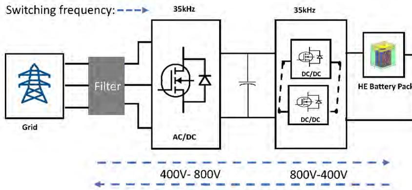
Figure 16. ZIG PE interface connecting the HE battery pack to the grid.
