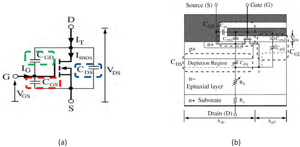
Figure 5. Intrinsic view of SiC Power MOSFET device (a) Internal equivalent capacitances (b) network outlook of cross-section area [1].
