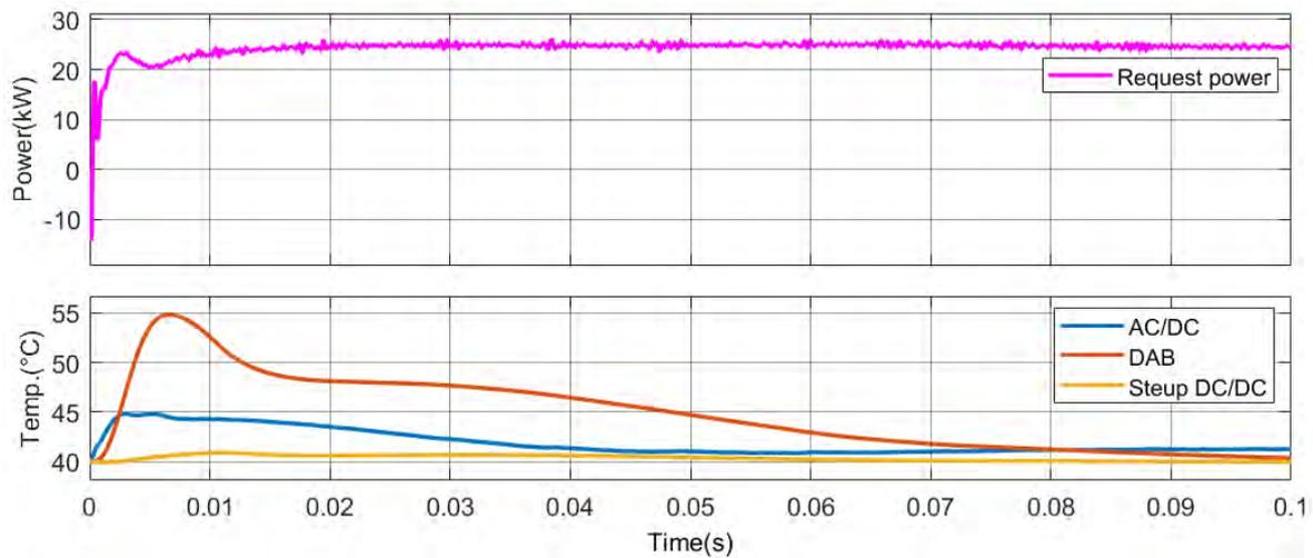
Figure 29. PT PE interface temperature dynamics in three stages.
