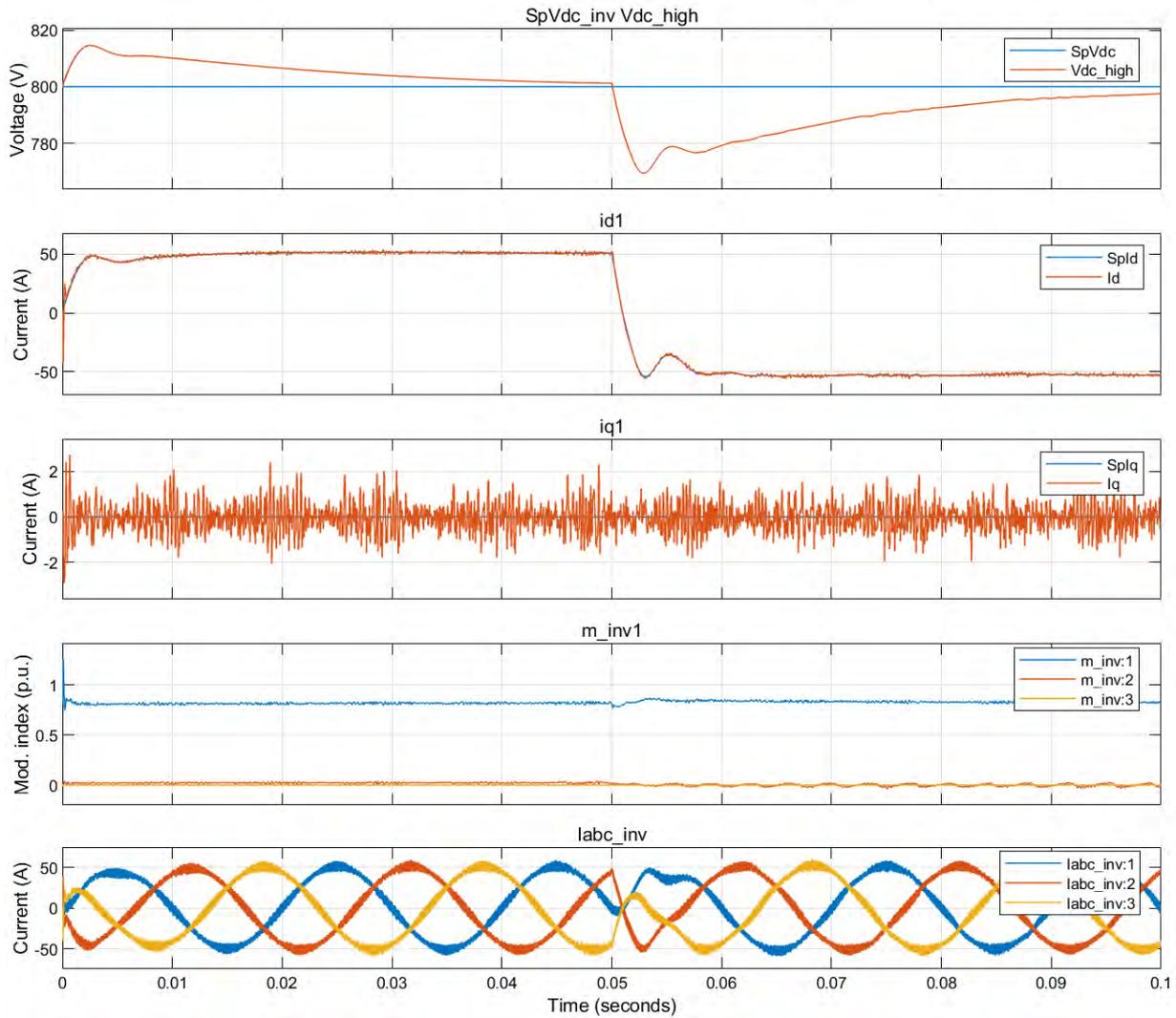
Figure 22. Some parameters of the inverter of the first PE module of HP branch.
