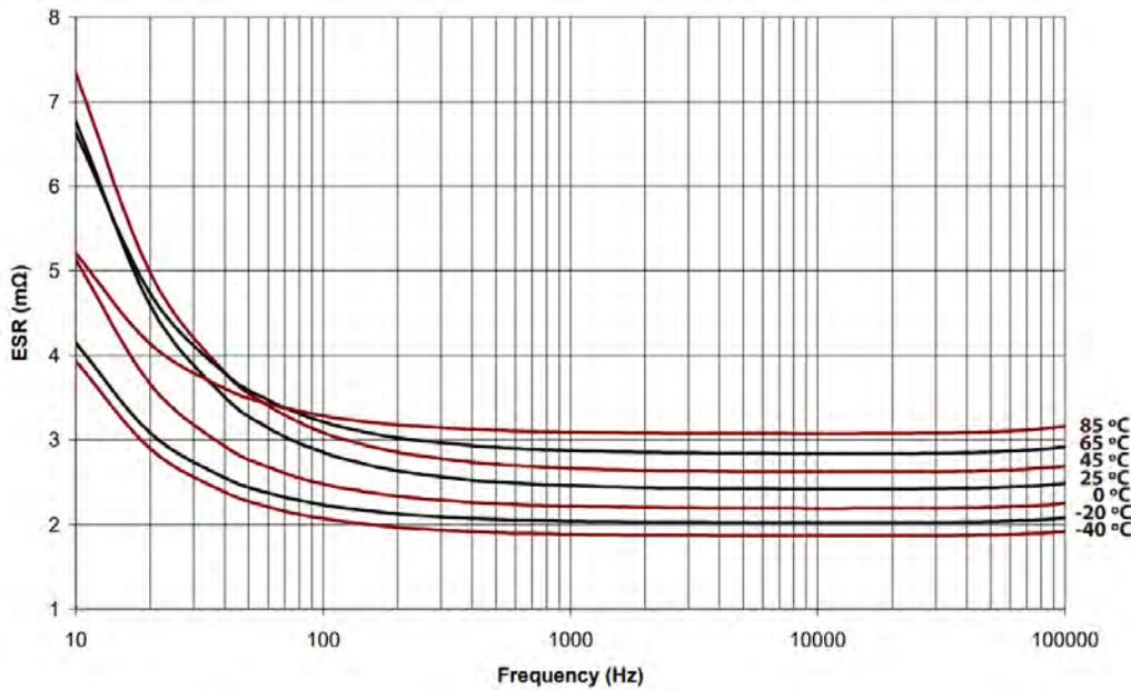
Figure 15. Behaviour of ESR as function of frequency and temperature.
