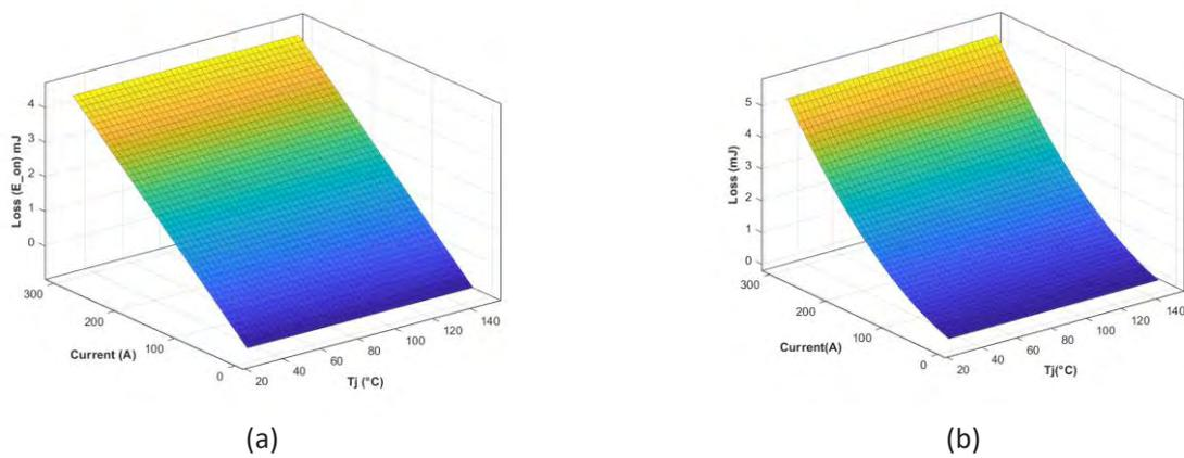
Figure 12. Switching losses for the low voltage regulation switch (S2).
