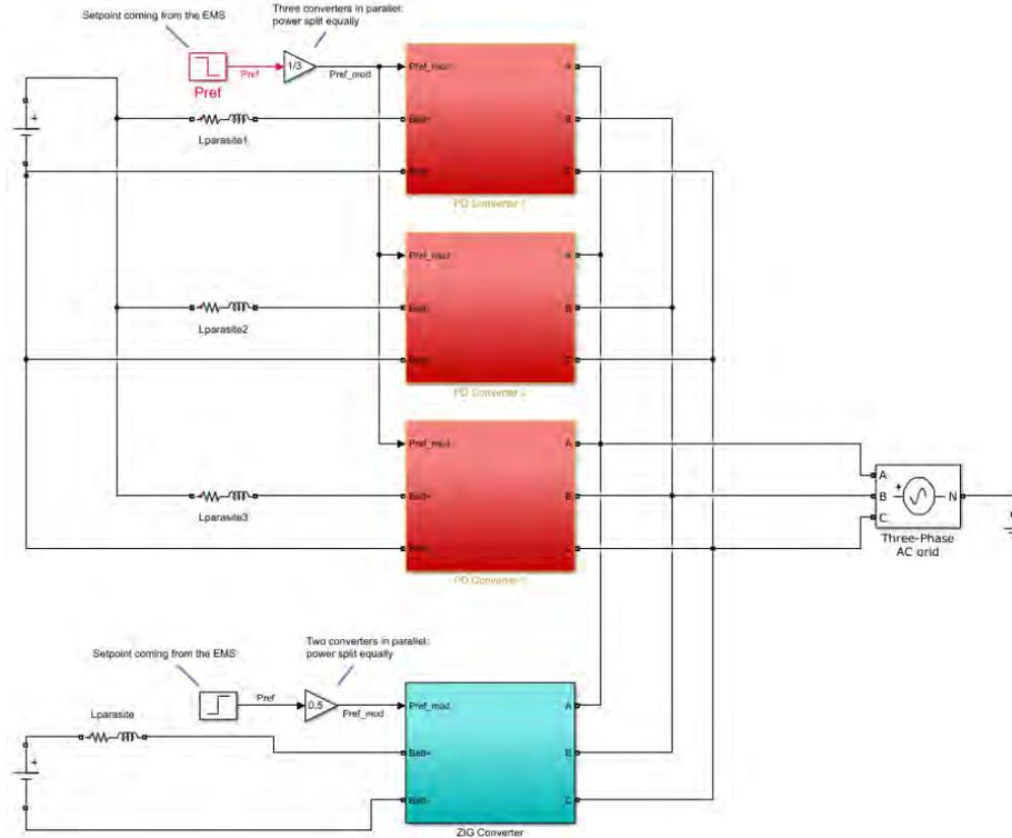
Figure 24. Complete converter simulation model to test the LLC
