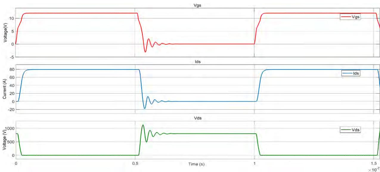
Figure 9. Dynamic characteristics of PT PE switch (S1) for  $V_{gs}$ ,  $I_{ds}$  and  $V_{ds}$ , tested at  $V_{ds}=800$  V,  $I_{ds}=80$  A and  $V_{gs}=12$  V.
