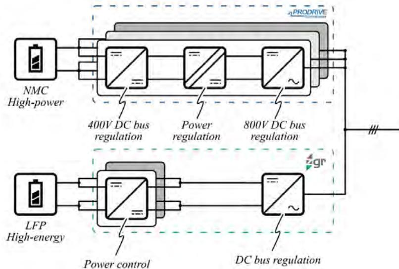
Figure 2. PE modules topology for both battery branches.
