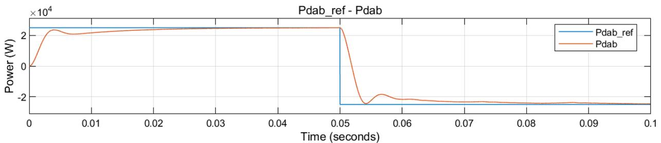
Figure 21. Active power step (in blue) and real active power (in orange) in the dual active bridge of the first PE module of HP branch.
