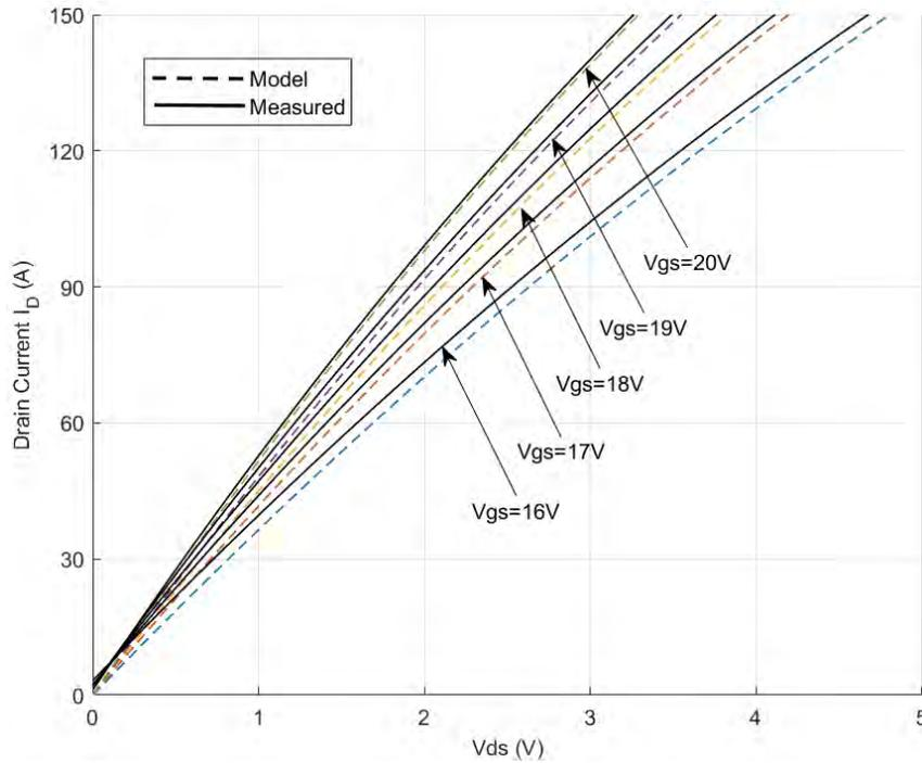
Figure 6. Drain current response with respect to drain voltage and different gate voltages at 25°C for S1.
