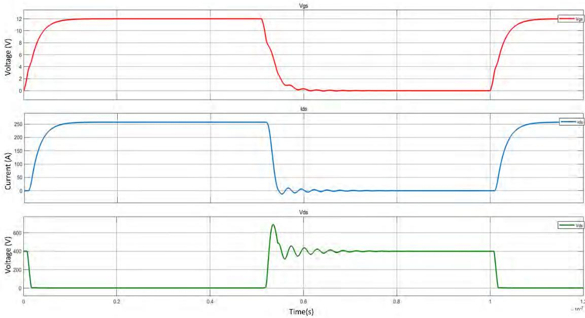
Figure 10. Dynamic characteristics of PT PE low side switch (S2) for  $V_{gs}$ ,  $I_{ds}$  and  $V_{ds}$ , tested at  $V_{ds}=400$  V,  $I_{ds}=250$  A and  $V_{gs}=12$  V.
