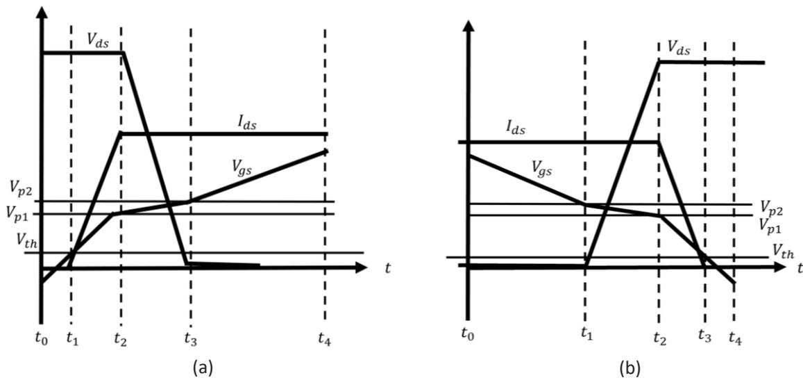
Figure 8. Switching timing sequence: (a) turn-on; (b) turn-off.
