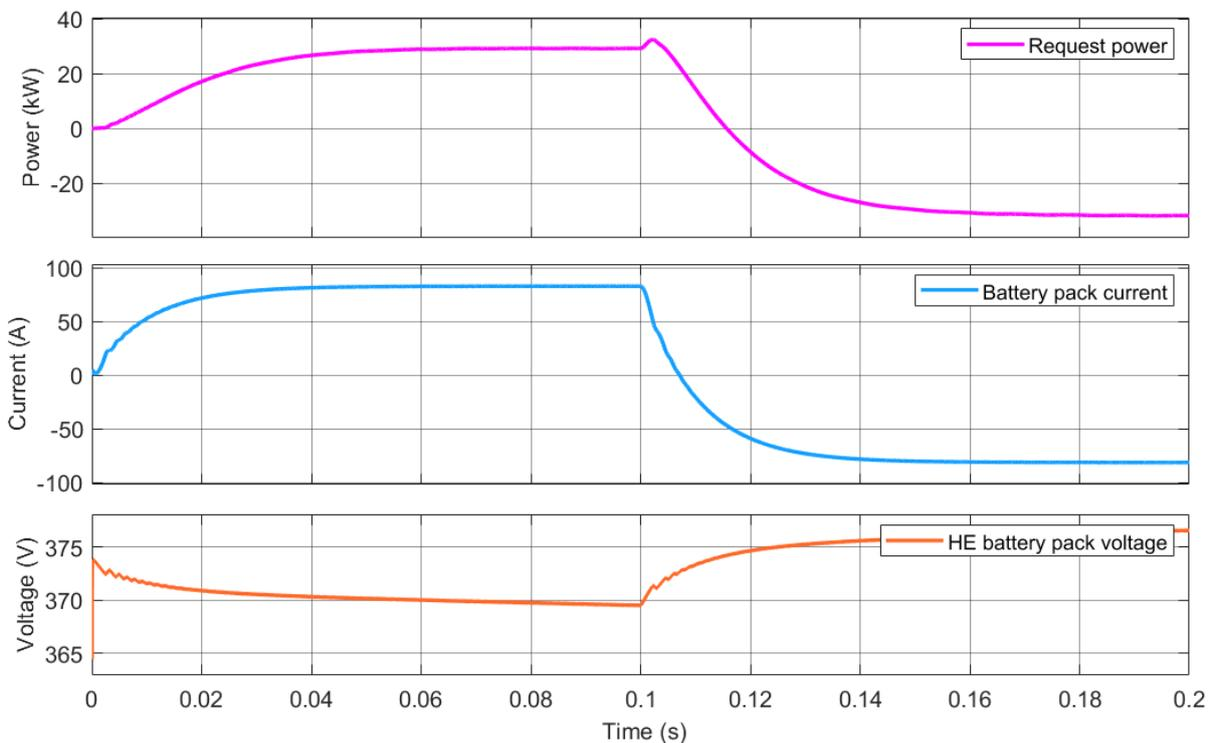
Figure 26. ZIG DC/DC power converter stage dynamics.
