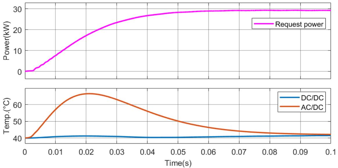
Figure 28. ZIG PE interface temperature dynamics.
