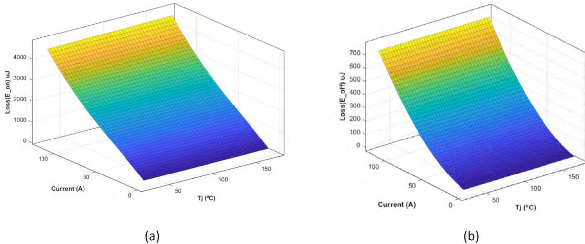
Figure 11. Switching losses for the high voltage regulation switch (S1).
