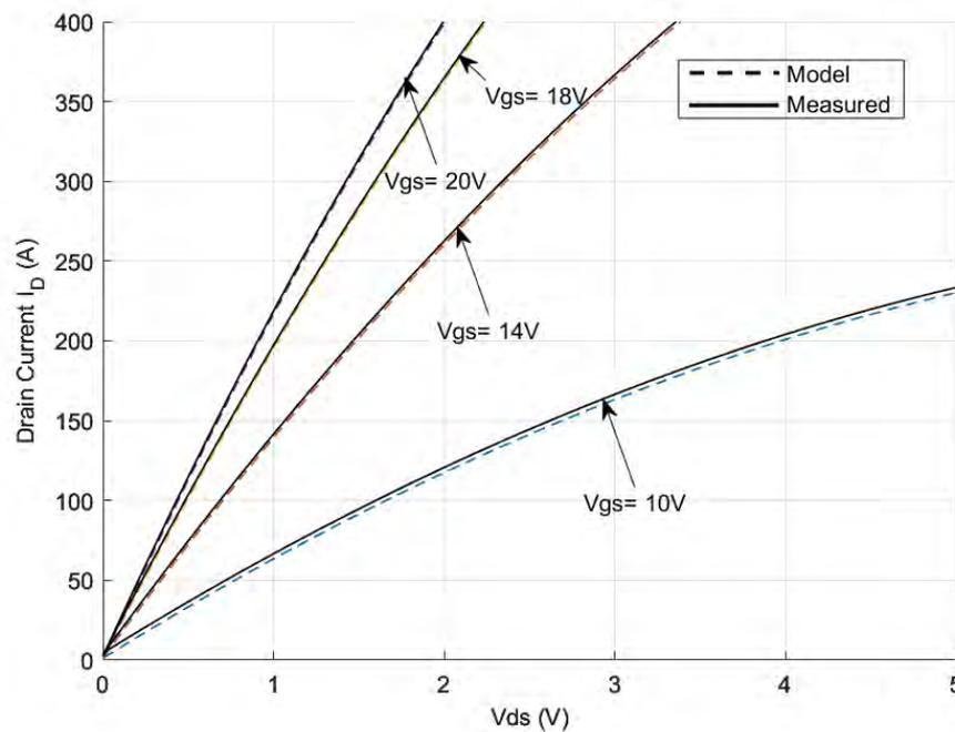
Figure 7. Drain current response with respect to drain voltage and different gate voltages at 25°C for S2: (a) excerpt of datasheet; (b) static model response.
